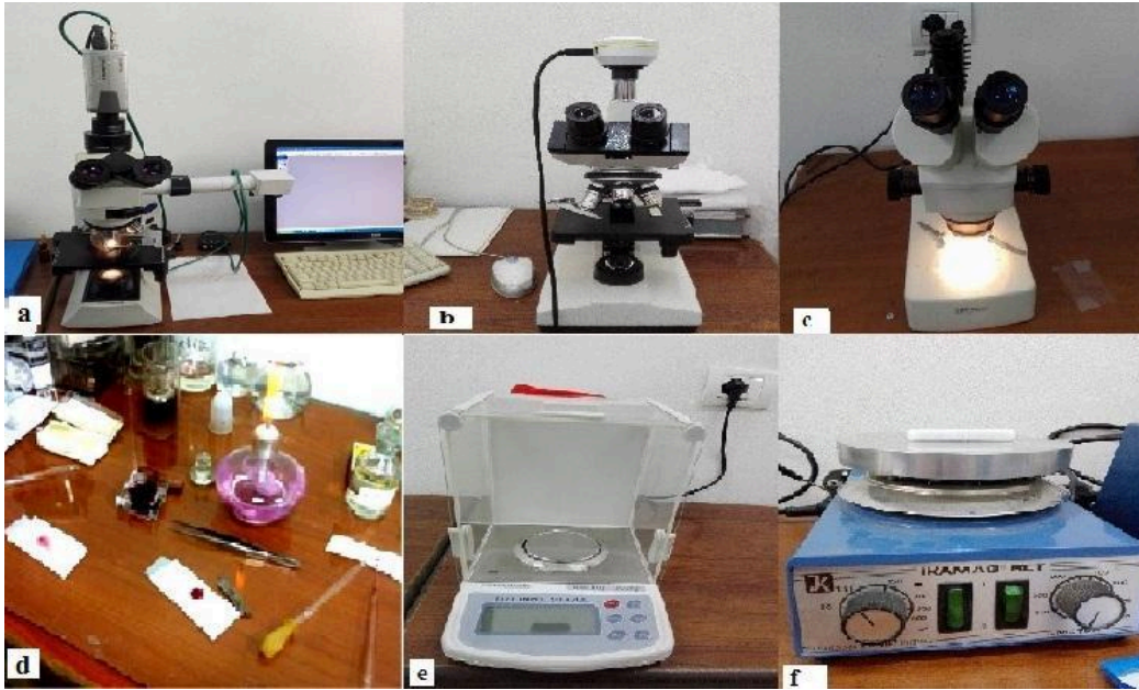
Fig. 1. Photo of the laboratory facilities and tools: a. Paralux trinocular microscope with Sony Paralux camera connected to a computer; b. Phase contrast microscope; c. Motik stereomicroscope; d. stainer and auxiliary equipment e. analytical balance and f. magnetic stirrer
